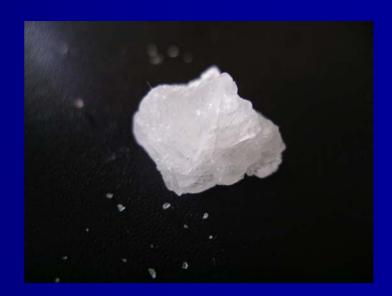
Impurities are only on the crystal surface. The salt is very well upgradeable with low losses.
