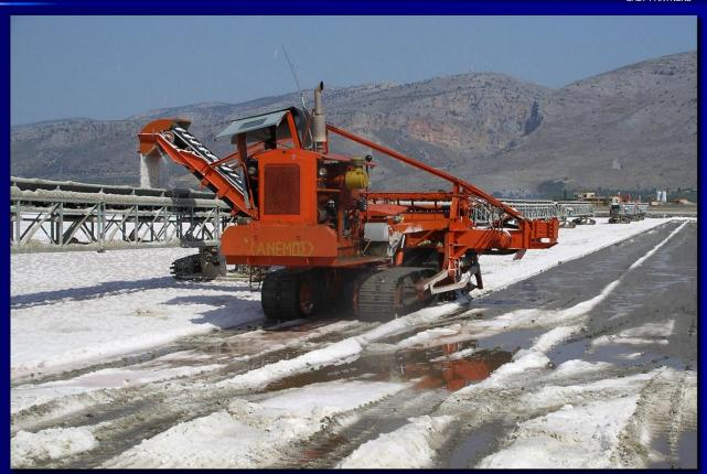
harvester drives on the crystalliser mud bed.
