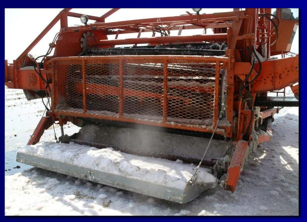
The cutting level is controlled mechanically by a plate sliding on the salt layer surface.
