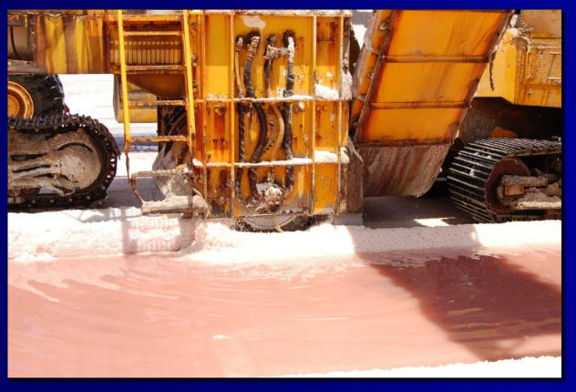
Salt is cut by a rotating drum upwards and discharged to a chain elevator located behind the drum.
