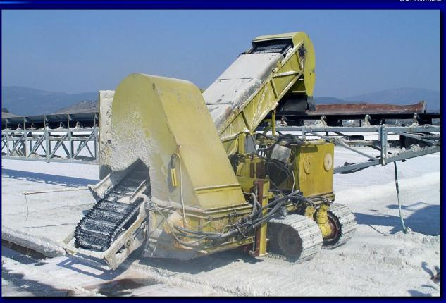
Kalloni saltworks operate a harvesting machine on Caterpillar tracks.
