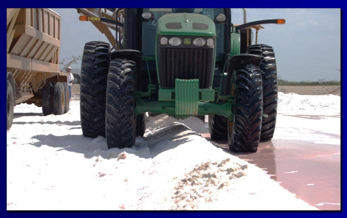
The salt layer is first ripped (scarified) and then windrowed.
