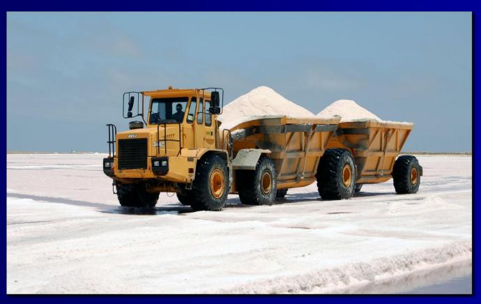
Wide wheel trucks with two trailers bring the salt from the harvester to the washing plant.
