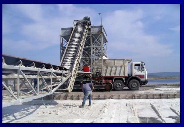
Belt conveyors bring the salt to a mobile bin driving on a causeway.
