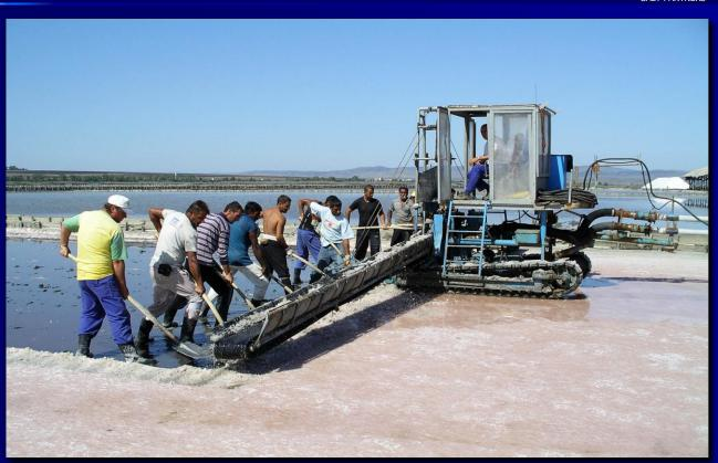
In Bulgaria, the transport of the harvested salt has been mechanised but the salt is still being harvested by hand.
