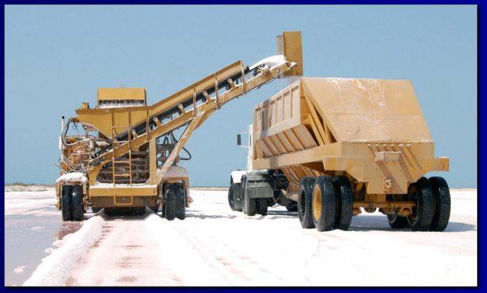
double wheels drives with one side on the salt and with the other side on the crystalliser bottom. The harvester lifts the salt to a double wheeled trailer pulled by a truck driving on the salt bed.
