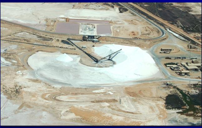
At Lake McLeod, the stockpile next to the wash plant has a design capacity of 1'500'000 t. In 2009 it was about 12% full.
