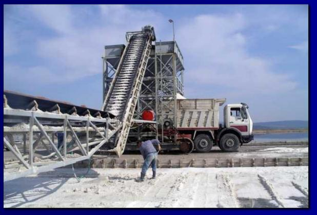
Belt conveyors bring the salt to a bin on wheels driving on a causeway. Lorries brine the salt to the washing plant.
