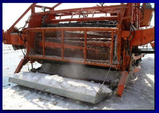
The cutting level is controlled mechanically by a plate sliding on the salt layer surface. The salt is broken upwards and lifted to a belt conveyor.
