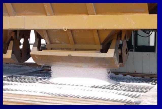
Salt is discharged from the trailers automatically, directly into the feeding hopper of the washing plant.
