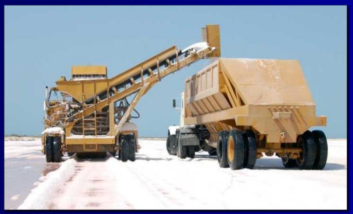
Tractor pulled harvester on double wheels drives with one side on the salt with the other side on the crystalliser bottom. The harvester lifts the salt to a truck pulled trailer, driving with double wheels on the salt.
