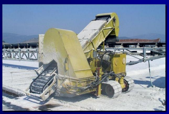
Kalloni saltworks operate a harvesting system consisting of a harvesting machine driving on the salt bed, cutting the salt on the side and lifting the salt onto belt conveyors has been in operation since many years.
