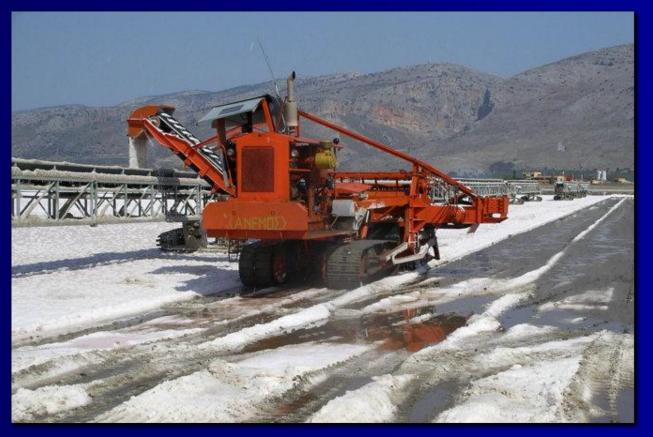
At Messolonghi, the harvester cuts the salt in front and drives on the crystalliser mud bed. It lifts the salt to a system of engine driven belt conveyors.
