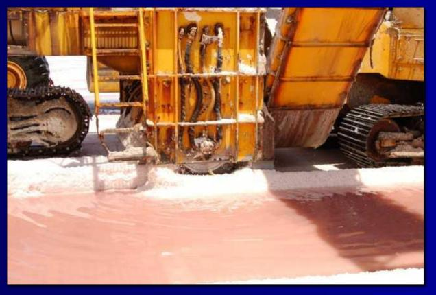
Salt is cut by a rotating drum upwards and discharged to a chain elevator located behind.
