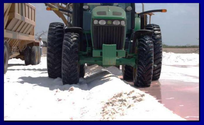
The salt layer is first ripped, then ploughed in a row. Salt floor is maintained on the crystalliser bottom. Cost of multiple operations is weighed against the cost of equipment.
